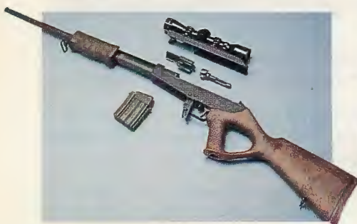
Ultra-short R6 carbine. To reduce the envelope to minimum possible dimensions, the gas block was moved rearward as far as possible and both the piston and gas tube shortened. Photo: courtesy LIW
